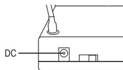
Insert the power adapter into the antenna's DC jack. Plug the other end into a wall outlet or power strip.
