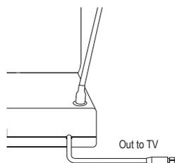
**Note:** If your TV's antenna input is already connected to a satellite receiver, cable box, or digital converter, connect the antenna's coaxial cable to the antenna input jack on that device.
