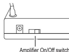
Set the amplifier on/off switch (on the antenna's back panel) to ON.
