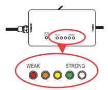
The signal meter on the antenna's amplifier measures the signal of the strongest UHF signal your antenna is receiving.
